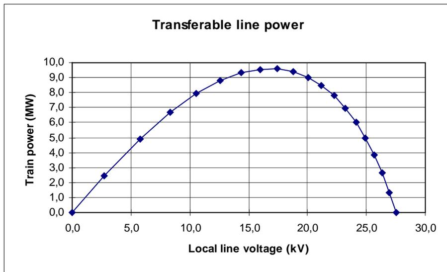
It is noticeable that an AC-AC vehicle cannot operate at the left side of the peak of the curve. This would create a positive feedback in the overall control loops, and cause a rapid collapse of the line voltage.
