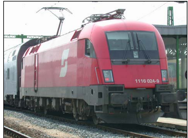
Figure 13. 6.4 MW locomotive (1.6 MW per traction motor), ÖBB class 1116, cf. figure 9. Photo by István Halász ( hihihihi@freemail.hu ) [12]
