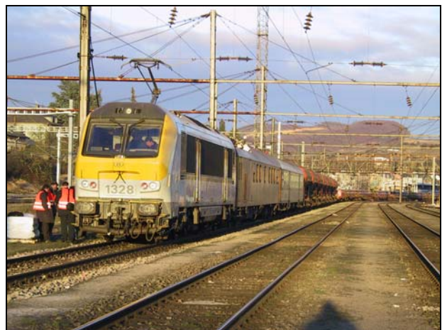
Figure 41. Tractive effort test, SNCB locomotive class 13 in Wasserbillig, Luxembourg. Photo by Paul Kettels, CFL
