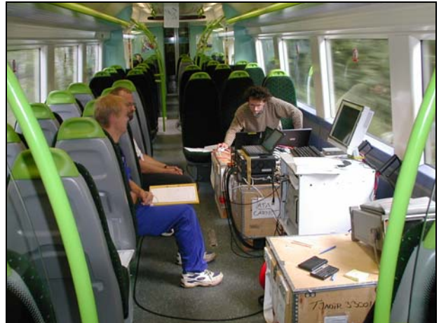
Figure 43. Interference Tests, Class 357 "Electrostar" EMU in Cerhenice, Czech Republic. Photo by Peter Mellberg, Bombardier Transportation
